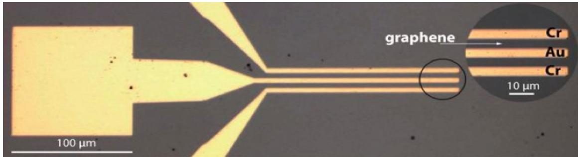
Top-down view of broadband, ultra-fast graphene detector capable of detecting terahertz frequencies at room temperature. (Cr = chromium, Au = gold).
